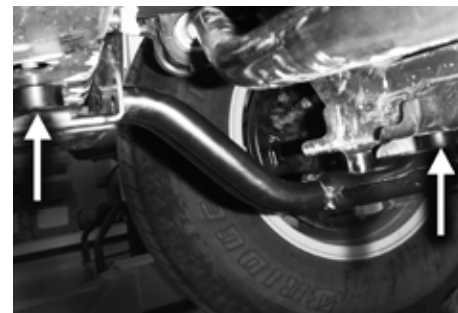
Fig. 6: Skid plate brace spacers
