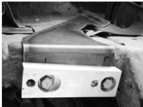
Fig. 3: Driver side sway bar relocation spacer
