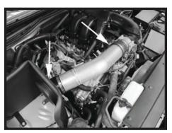
Step 16 Install the end of the intake tube into the reducer coupler on the throttle body. Install the velocity adapter in the heat shield and onto the angled coupler. Once the tube is in the desired location, tighten all the clamps.
