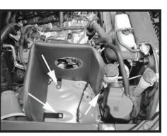
Step 14 Install the heat shield into the truck as shown with the supplied hardware and the bolt removed in Step 13.
