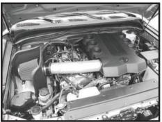
Reinstall the engine cover. Make sure that all clamps and hardware are fully tightened. Reconnect the battery cable, start the vehicle
