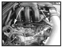
Step 17 Install the fuel pressure vent line from the fuel pressure regulator to the small vent tube on the intake tube. Reconnect the crank case vent line.
