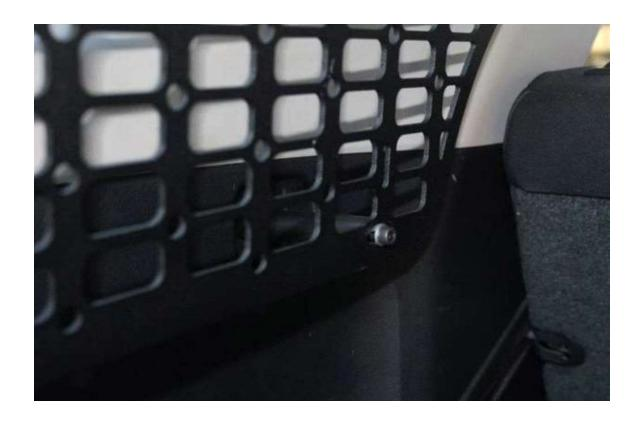
8. Use the slack in all your bolts to even up the PSD rack to be even across the top of your window opening. The PSD rack is made to have plenty of adjustment to make this easier.
