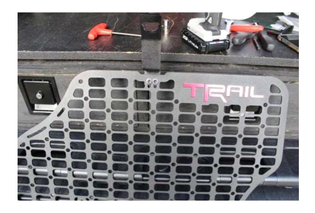
3. Remove the Upper coat hook from your 5th Gen 4 Runner. Use the 10 mm Socket set. Keep
