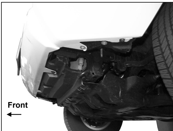
(Fig 1) Remove hardware attaching bottom of plastic bumper cover
