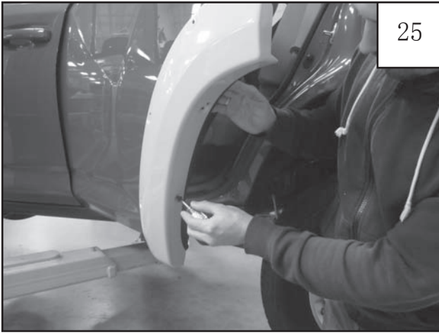
Install supplied Truss Head Screws (SW1-0044) into holes. Screws are attached to factory flare. DO NOT OVER TIGHTEN SCREWS.
