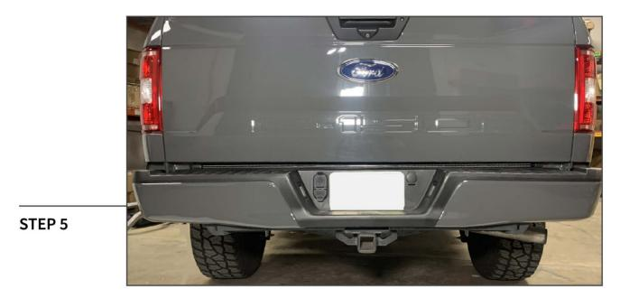
Plug the LED tailgate bar connector into the vehicle 4-pin trailer wiring plug. Note: Using the provided scotchloks, the LED tailgate bar can be spliced into the trailer wiring behind the bumper.
