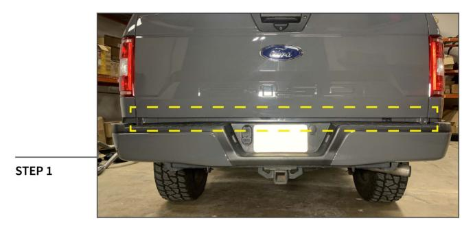
Using the provided (1) alcohol prep pad, clean the area under the tailgate on the vehicle. Once dry, use (1) adhesion promoter pad to prepare for tape adhesion.
