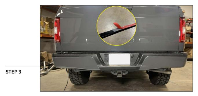
Route the attached wiring behind the rear bumper. Align the LED tailgate bar to the vehicle and familiarize the fitment to the vehicle. Peel the red tape backing and adhere the LED tailgate bar to the vehicle. Apply firm pressure to ensure proper adhesion.
