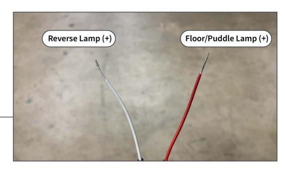
Wire the (2) separate wire leads to the vehicle lighting using the diagram below. Splice each connection using the provided (2) Scotchlok connectors.
