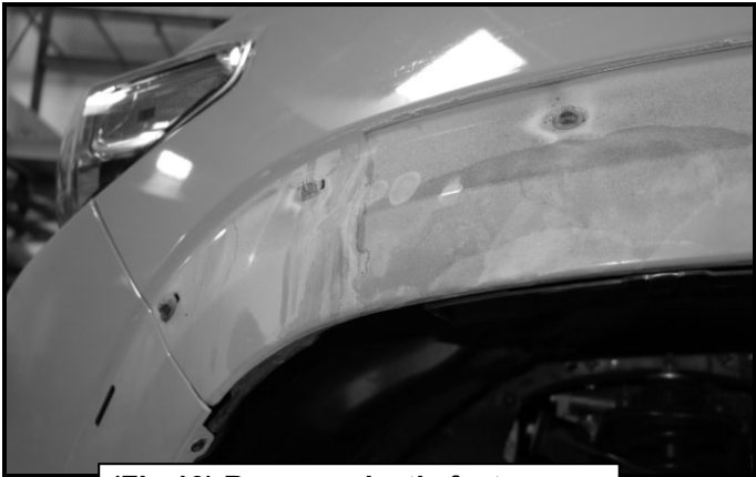
(Fig 10) Remove plastic fasteners
