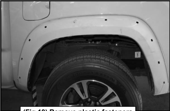
(Fig 18) Remove plastic fasteners
