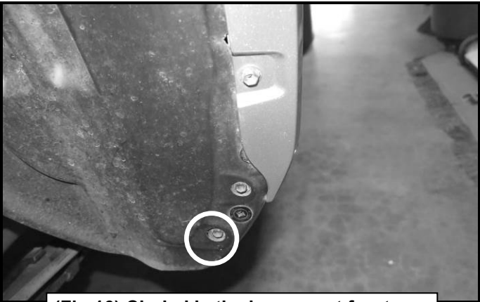
(Fig 16) Circled is the lowermost front bolt which will need to be saved for later
