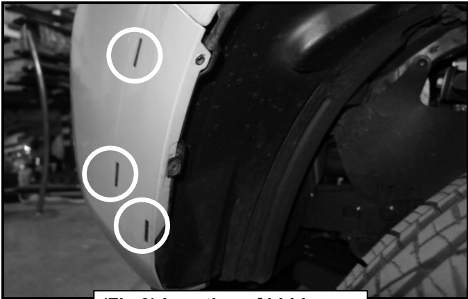
(Fig 9) Location of hidden fasteners
