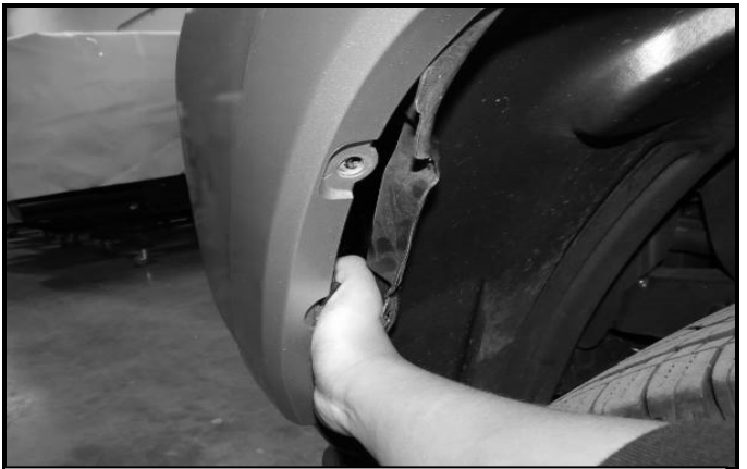
(Fig 8) Insert hand behind this section to release hidden fasteners
