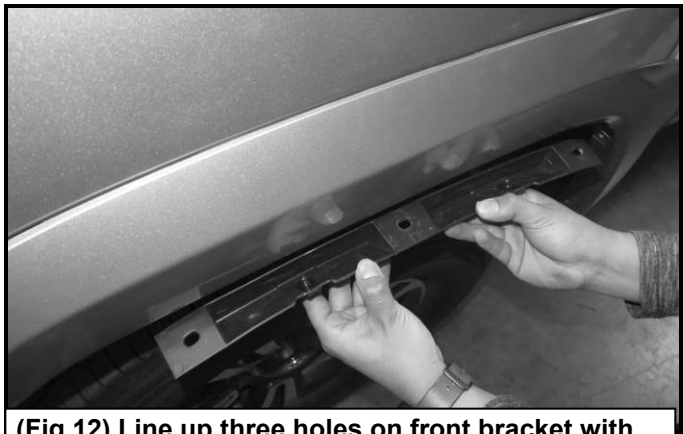
(Fig 12) Line up three holes on front bracket with three uppermost mounting holes on the vehicle. Note the direction of the bracket and the "U" clips
