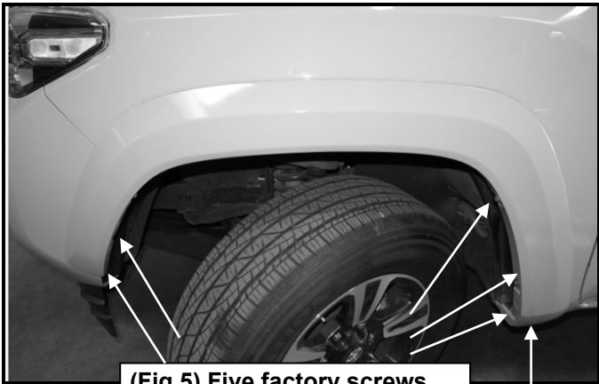
(Fig 5) Five factory screws, driver's side front
