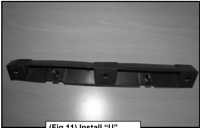
(Fig 11) Install "U" Clips
