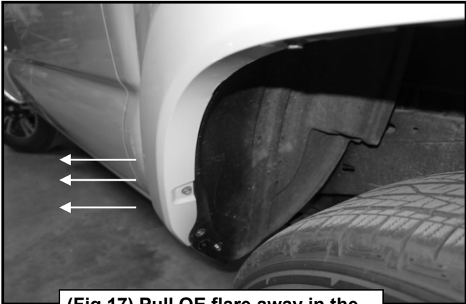
(Fig 17) Pull OE flare away in the direction shown
