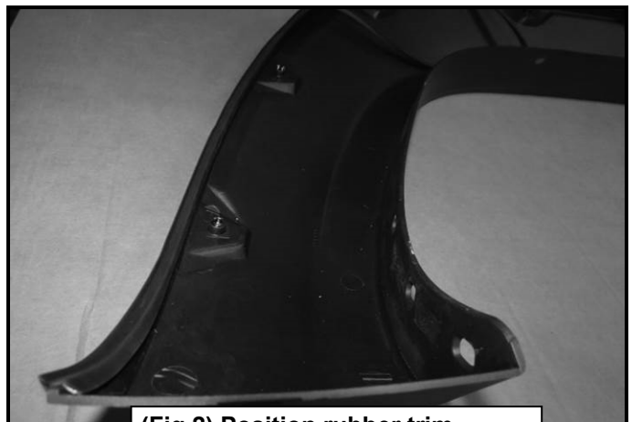
(Fig 2) Position rubber trim correctly with the wiper side on the outer surface of the flare
