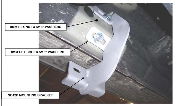
**STEP 3.** Loosely attach one of the NO42P mounting brackets to the body using the 8mm x 25mm hex bolts, 8mm hex nuts, 5/16" flat washers and 5/16" lock washers as shown. Repeat the procedure for the passenger side center and rear brackets.
