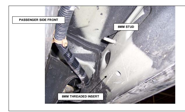
**STEP 2.** This installation uses three mounting brackets per side. Begin by installing the passenger side front mounting bracket. Locate the stud and threaded insert in the under side of the body. Note: you may need to remove the plastic plug to expose the threaded insert.
