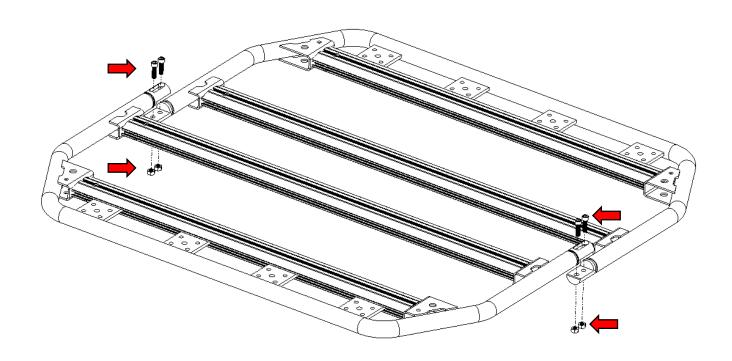
Place the sections so the coupling joint matches each other. Secure each side using (2) 5/16" allen socket bolts and (2) 5/16" hex nuts.
