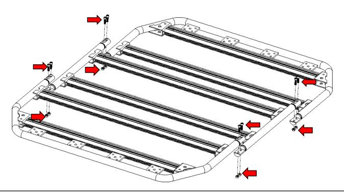
• If you want to extend the rack use a connecting center (sold separately). Place the sections so the coupling joint matches each other. Secure each section using (2) 5/16" allen socket bolts and (2) 5/16" hex nuts.
