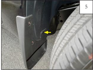
Remove (1) factory push fastener. Remove and discard mudflap.
