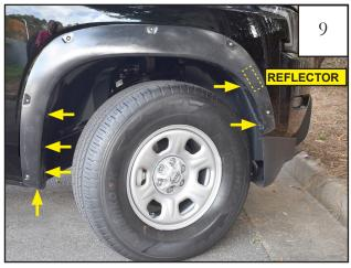
Reinstall (6) factory screws. Apply side reflector (LT1-0002). Front flare installation complete.
