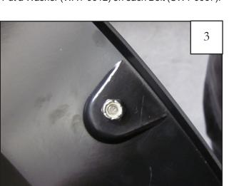
Place a Nut (NU1-0019) over the end of each Bolt and tighten, using a 1/2" wrench for the Nut and the supplied Torx Bit (SW1-0052) for the Bolt. Repeat for remaining pockets.
