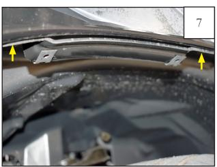
Install bracket using using (2) previously removed screws.
