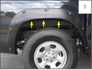
**NOTE:** For long bed installation only: Hold flare in position and mark (3) locations where holes in flare align with truck fenderwell. Mark these locations with a grease pencil. Proceed to **Step 6**.
