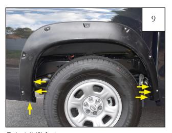
Reinstall (6) factory screws. Rear flare installation complete. Repeat for opposite side.
