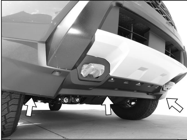
(Fig 1) Model with splash guard (arrows)
