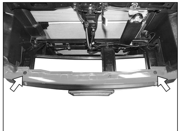
(Fig 9) Remove fasteners attaching top of bumper cover to steel bumper brackets (arrows)
