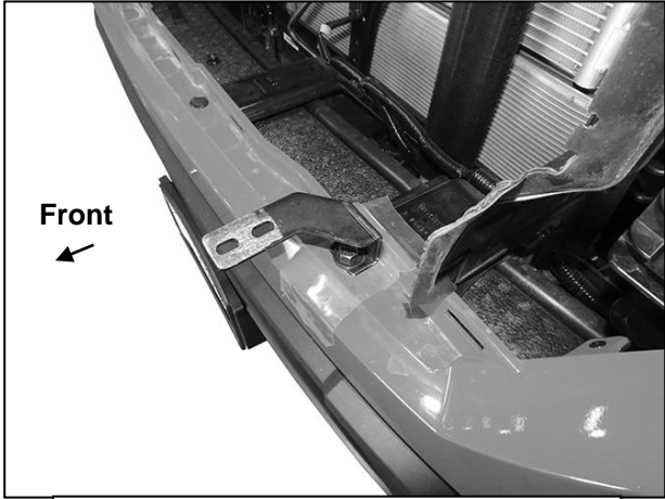
(Fig 11) Attach driver/left side Inner Top Mounting Bracket to top of bumper
