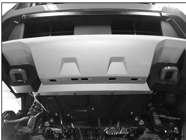
(Fig 5) Remove tow hooks if equipped. PRO4X model not equipped with splash guard pictured from below
