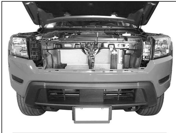
(Fig 8) Remove factory grille assembly
