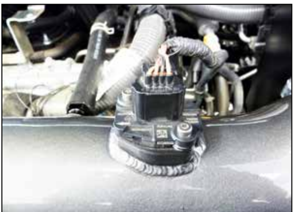
18. Reconnect the mass air sensor electrical connection.
