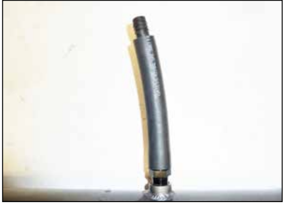
14. Assemble the CCV hose onto the K&N intake tube as shown.
