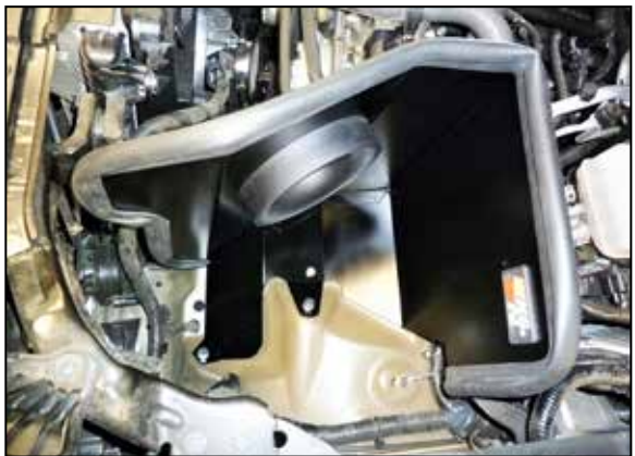
11. Install the heat shield into the vehicle and secure with the provided hardware.
