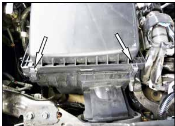
5. Release the spring clips that secure the upper air filter housing and then remove the upper housing and intake tube from the vehicle.
