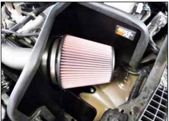
19. Install the K&N air filter and secure with the provided hose clamp.
