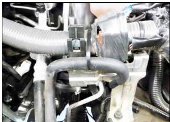
8. Use the provided tie wrap to secure the front differential vent to wiring harness as shown.
