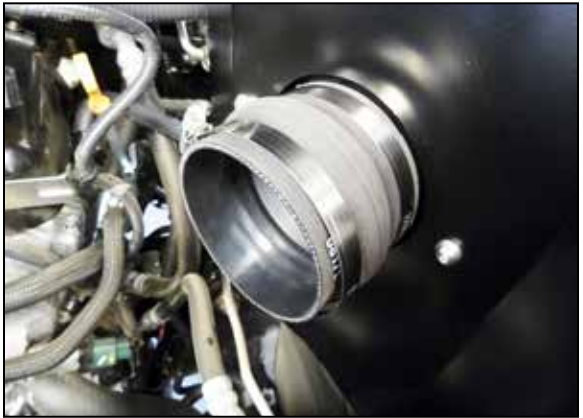
12. Install the provided hump coupler onto the filter adapter using the provided hose clamp.
