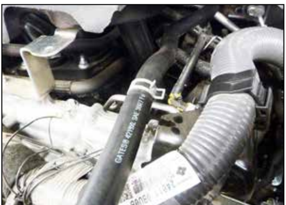
17. Connect the factory CCV hose to the Assemble K&N CCV hose.
