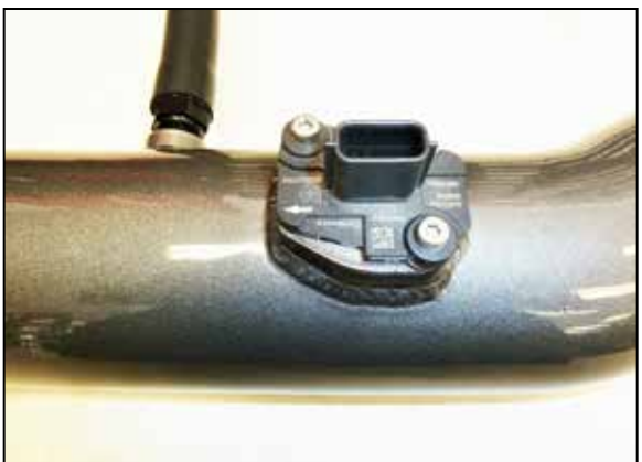
15. Remove the mass air sensor from the factory housing and install it into the K&N intake tube using the provided hardware.
