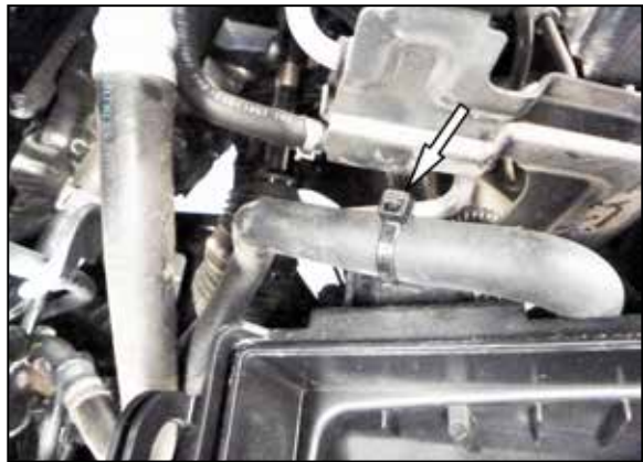
6. On 4X4 equipped vehicles, cut the tie wrap that secures the front differential vent line to the lower air filter housing. Lift the lower housing up and remove it from the vehicle.
