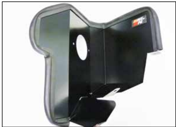
9. Install the provided edge trim onto the heat shield as shown. Install the K&N badge into the heat shield and lock with the provided locking plate.
