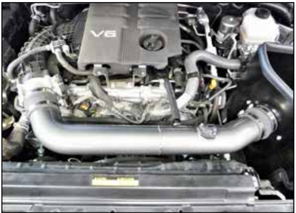
16. Install the K&N intake tube into the couplers, adjust for best fit and secure the hose clamps.
