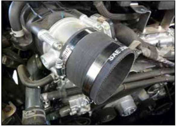
13. Install the straight coupler onto the throttle body and secure with the provided hose clamp.
