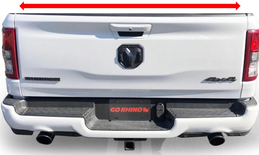
Measure the inside bed rail distance. Use that distance to determine the spacing for the SRM towers.
