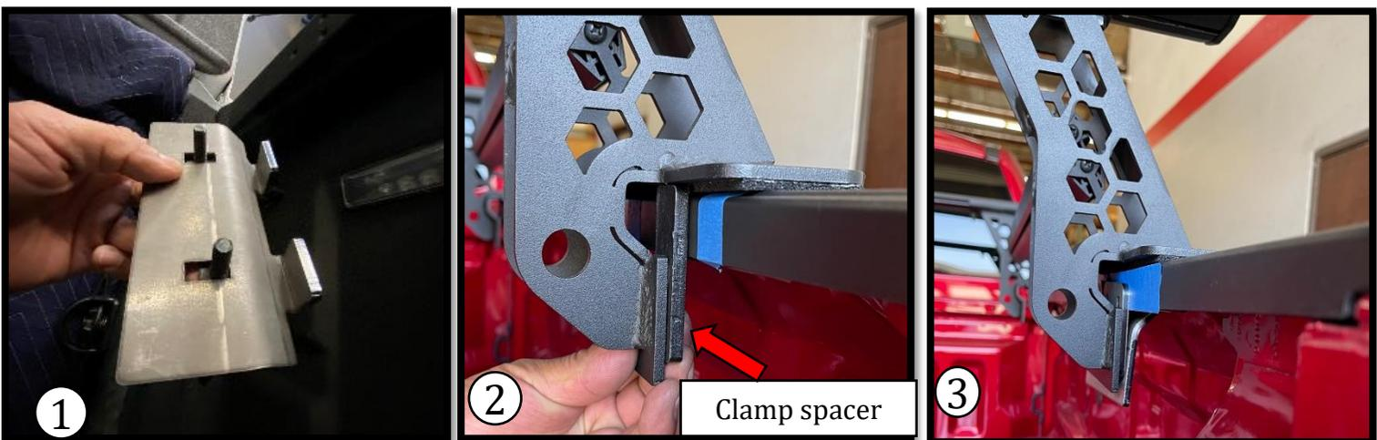
Use the provided bed rail clamp and install 5/16" carriage bolt from the backside (image 1). Place clamp spacer plate onto the bed rail clamp so that it acts as a spacer to square the clamp against the inside of the bed rail (image 2). Once the threads are exposed, position the clamp against the inside of the bed rail and use 5/16" flat washer, 5/16 lock washer, and 5/16 hex nut to secure the clamp. Leave finger tight for final adjustment. Repeat process for each corner.
