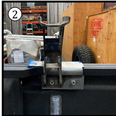
Use the provided bed rail clamp and install 5/16" carriage bolt from the backside (image 1). Once the threads are exposed, position the clamp against the inside of the bed rail and use 5/16" flat washer, 5/16 lock washer, and 5/16 hex nut to secure the clamp (image 2). Leave finger tight for final adjustment. Repeat process for each corner.
