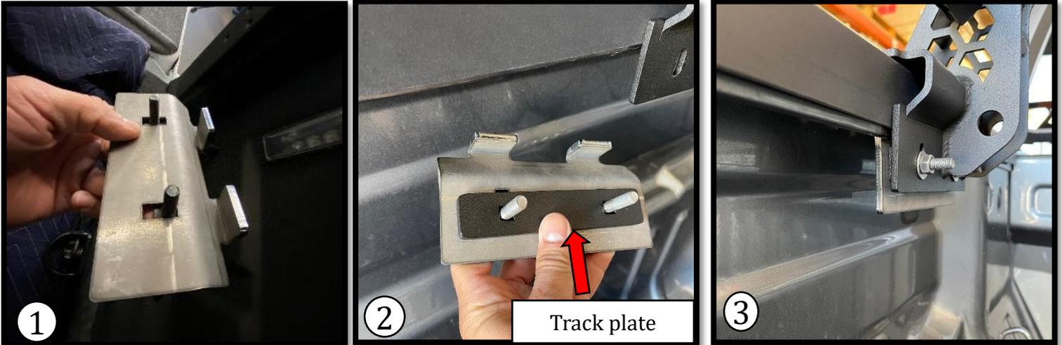
Use the provided bed rail clamp and install 5/16" carriage bolt from the backside (image 1). Place track system plate onto the bed rail clamp so that it acts as a spacer to square the clamp against the inside of the bed rail (image 2). Once the threads are exposed, position the clamp against the inside of the bed rail and use 5/16" flat washer, 5/16 lock washer, and 5/16 hex nut to secure the clamp. Leave finger tight for final adjustment. Repeat process for each corner.
