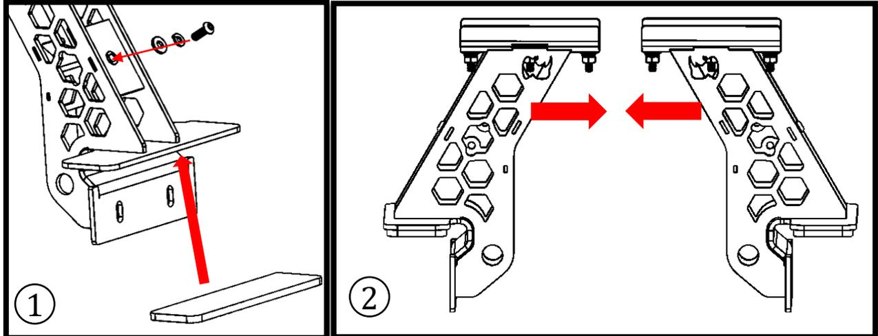
Install foam adhesive on the mounting surface of the SRM tower (image 1). Install  $\frac{1}{4}$ " button head screw,  $\frac{1}{4}$ " lock washer,  $\frac{1}{4}$ " flat washer onto the threaded riv-nut. Repeat steps for all four towers. Position each tower mounted be sure the Rhino heads are facing each other (image 2).
