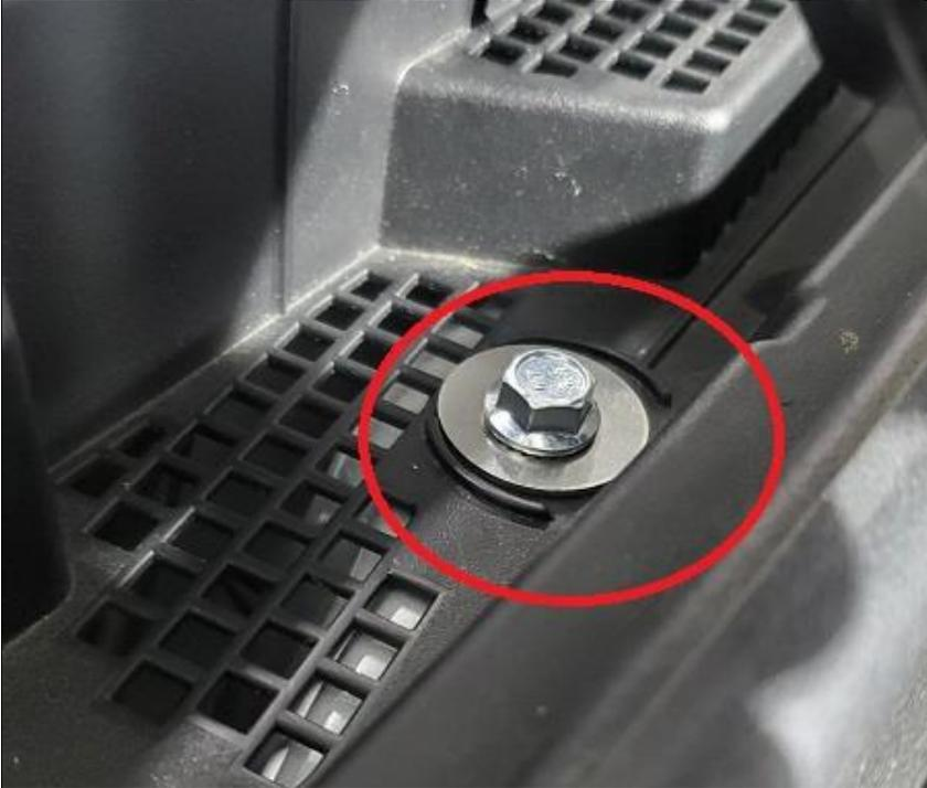
Now take J&L mounting bracket and slide it over the bolt that came through the bottom of the cowl. Use supplied nut to secure bracket but do not tighten bolt completely yet
