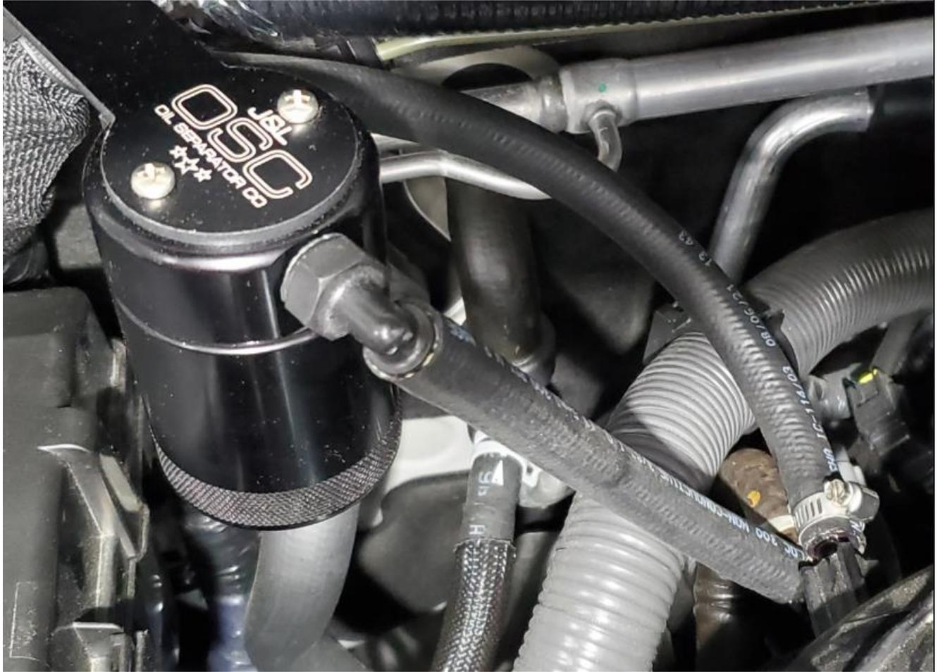
**6** Once hoses are connected, tighten mounting bracket bolt.
