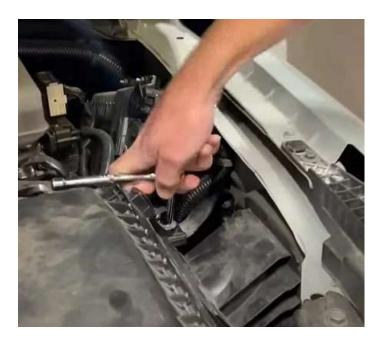
Loosen the hose clamp on the throttle body.
