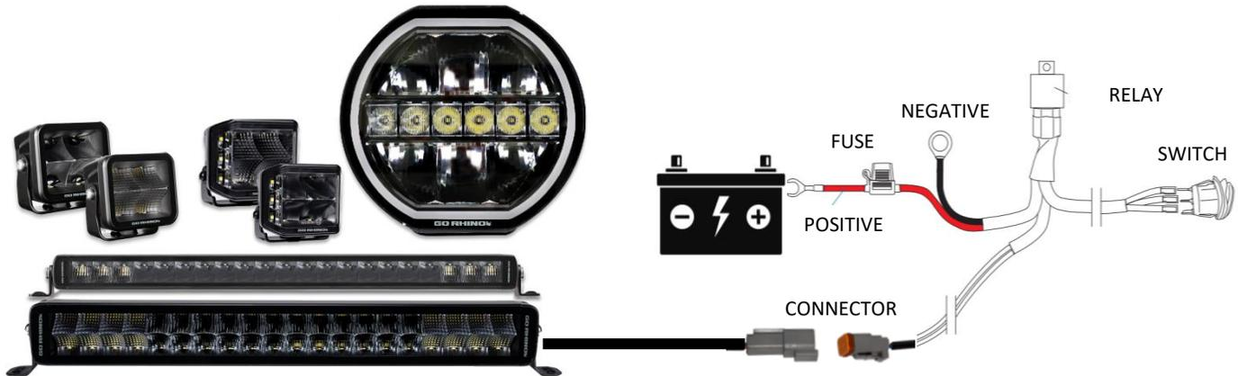
STEP 1: When routing wire harness through any metal surface be sure it is free of any sharp edges and protected using wire sheathing or a grommet.
