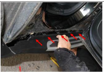
5. Adjust the T-Bolt2" to insert it into the hole of the bracket; Push the pedal to tighten the lower nut slightly.
