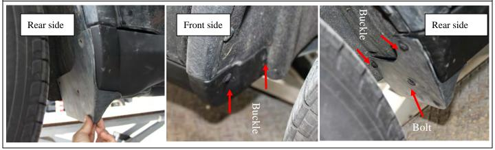
8.Take the M6 self tapping screw for fastening and the position below the mudguard as shown in the diagram.
