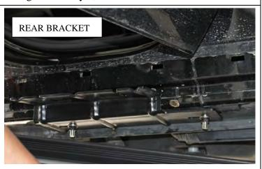
4. Put "T-Bolt 2" on the profile on the back of the pedal and put 4 bolts in each card slot to make it correspond to the hole position of the support; At least two people lift the pedal to align its bayonet with the body hole, confirm and push in.
