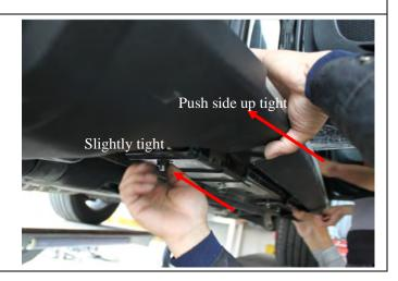
6. Check whether the pedal and the body are installed properly. Push and tighten the nuts of the profile and iron bracket after the installation is in place, and then tighten the nuts of the iron bracket on the body, as shown in the figure.
