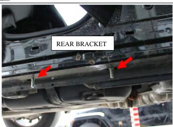
3. Place the front and rear brackets, flat washers, and spring washers at the corresponding positions of the T-bolts, and then tighten the flange nuts slightly. Do not tighten them yet, and fix the brackets.
