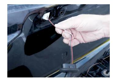
**Step 11:** Take the new camera panel, slide in the white connector in the hold you just pulled the old one out of, push till you hear the small white clip snap into place.
