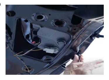
**Step 5:** There are eight silver 10mm nuts between the taillights that need to be removed as they're holding the exterior panel on.
