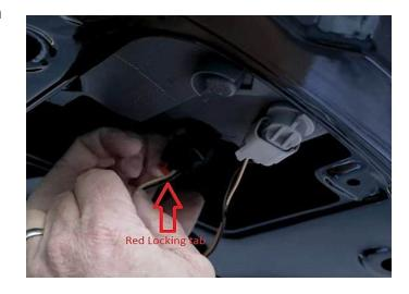
**Step 8:** You can now push in the tab on the inner part of the taillight to release the taillight.
