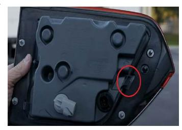
**Step 9:** Time to remove the factory panel from the rear of the vehicle. Use some needle nose pliers to pinch the white tab that is left holding the panel in place.
