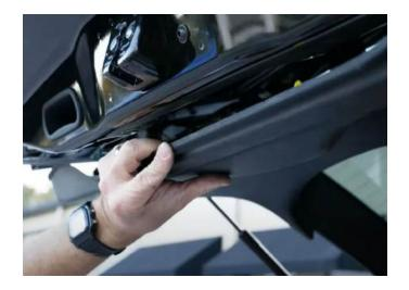
**Step 2:** Disconnect the two connections to the panel. Push the locking tab over to disengage the connection.
