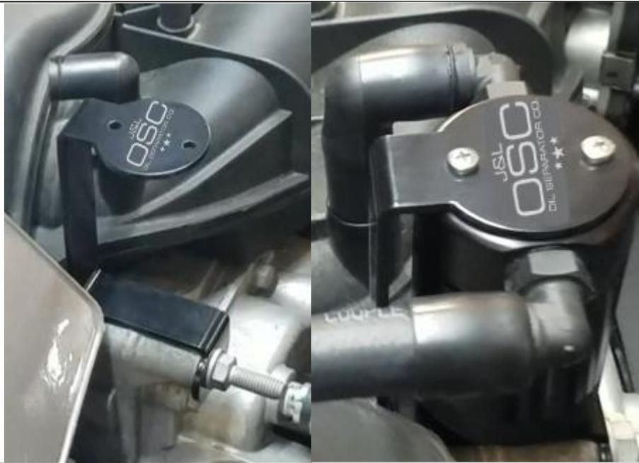
Use light oil on the fitting into rubber connector on intake manifold (near PCV cap)
