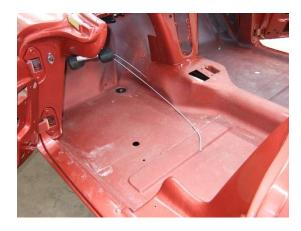
Remove the seats, carpet and trim panel sections surrounding the firewall and tunnel on both driver and passenger side. Remove carpet pad and any loose foam pieces down to the firewall surface. There no need to remove factory damping material unless it is delaminating or flaking. If it is delaminating or flaking just remove the loose pieces.
