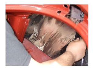
Start at one straight edge (side or top of the firewall as far under the instrument panel as you can reach). If a ground up restoration and no trim or instrument panel is in vehicle – start at the top of the firewall just under the windshield frame. If the instrument panel is installed reach up to the base of the instrument panel.
