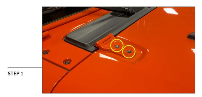
Remove (2) T-50 Torx bolts from the hood hinge.
