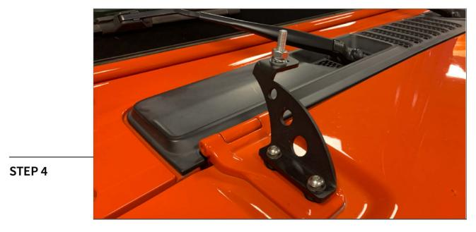
Insert (1) M10 x 40mm stud through the bottom of the hood mount. Secure the stud in place using (1) M10 flat washer, (1) M8 lock washer, and (1) M10 nut. Tighten until secure.
