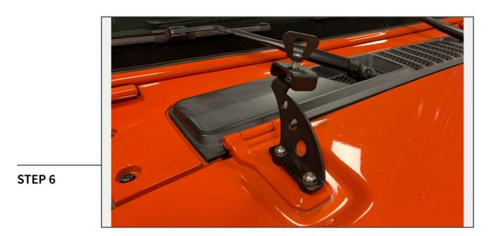
Place the jack onto the hood mounts. Once placed, install (1) hold down bracket over the jack on each side of the vehicle. Secure the jack using (1) wing nut per hood mount. Use the supplied strap to secure the jack closed.
