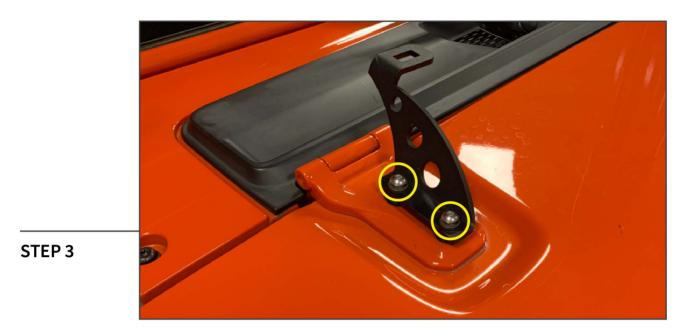
Place (2) conical spacers in the original bolt holes in the hood hinge. Place the hood mount onto the spacers, then secure the hood mount to the vehicle using (2) M8 x 35mm Allen bolts, (2) M8 lock washers, and (2) M8 flat washers. Tighten until secure.
