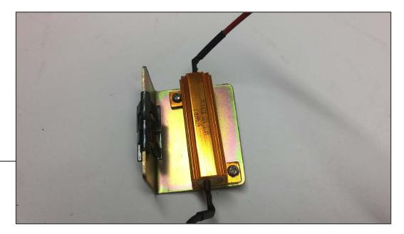
Using (2) clips per side, clip the resistor bracket to the vehicle.
