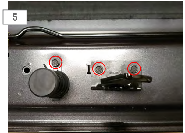
Remove the (2) 10mm hood latch bolts, and (1) 10mm hood stopper bolt. Remove both the hood latch and the hood stopper. Transfer both the hood latch and the hood stopper to the new hood using the factory hardware.
