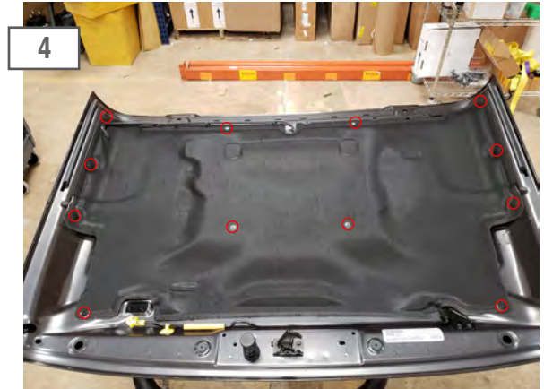
Using a trim panel removal tool, remove the (12) plastic push pins securing the hood liner to the hood. Remove the hood liner.
