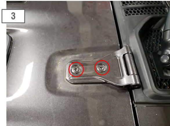
Using a T50 torx bit, carefully unbolt the hood hinges from the hood. With a helper, carefully remove the hood and place upside down on a non abrasive surface.
