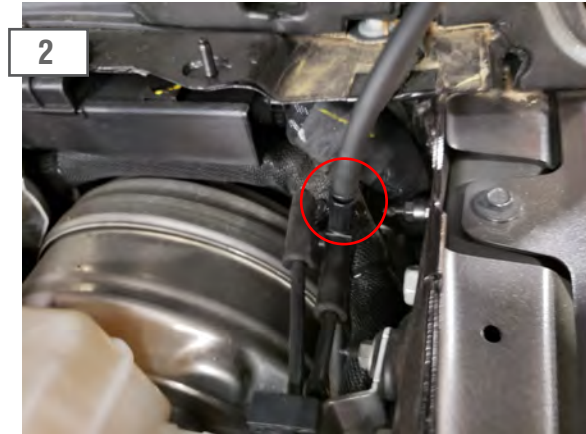
Next, lift the hood to locate the windshield washer fluid hose connection. Disconnect the hose connection.
