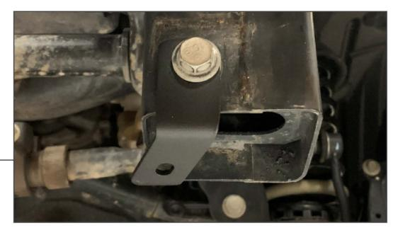
Loosely install the (2) skid plate brackets to the vehicle's original skid plate mounting location using (2) original vehicle skid plate bolts.
