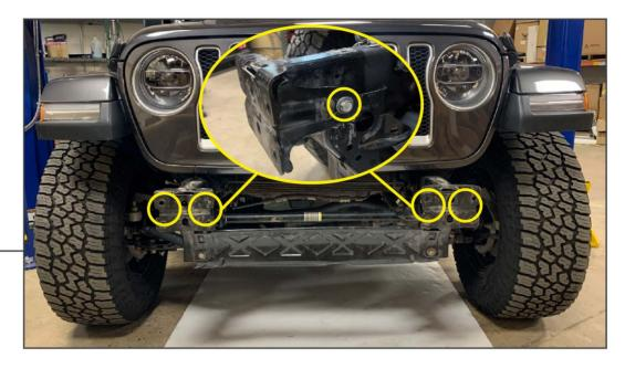
Remove (4) 16mm bolts to remove the inner and outer bumper support brackets.
