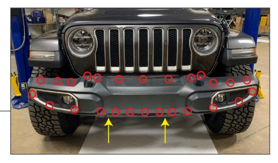
Remove all the plastic push clips from the backside of the bumper using a panel removal tool. Use the (2) 8mm bolts from the bottom of the plastic splash shield under the vehicle.
