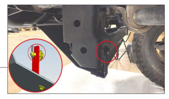
Loosely install the (2) skid plate brackets to the vehicle's lower radiator support using (1) M8 x 35mm stud plate, (1) M8 lock washer, (1) M8 flat washer, and (1) M8 nut per side.
