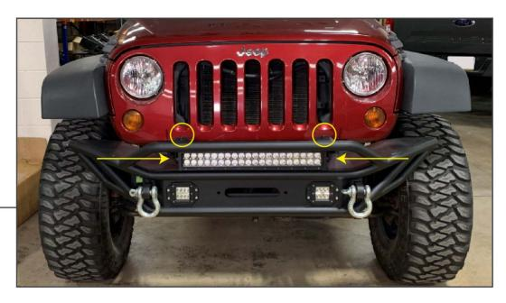
Secure the light bar bracket to the bumper using (2) M8 x 25mm Allen bolts, (2) M8 lock washers, (2) M8 flat washers, and (2) M8 nuts. Secure the light bar to the brackets using (2) M8 x 16mm Allen bolts, (2) M8 lock washers, and (2) M8 flat washers. Using the provided wiring harnesses, connect the lights to the vehicle.
