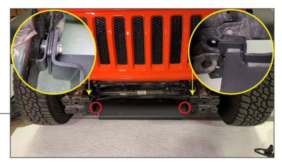
Align the winch plate in between the vehicle frame rails. Install (1) 8mm spacer on the driver side, and (2) 3mm spacers on the passenger side in between the winch plate and the frame rail. Install the bottom of the winch plate to the frame using (1) M12 x 130mm bolt, (1) M12 lock washers, (2) M12 flat washers, and (1) M12 nut per side. Insert the bolts through the frame rail and winch plate.
