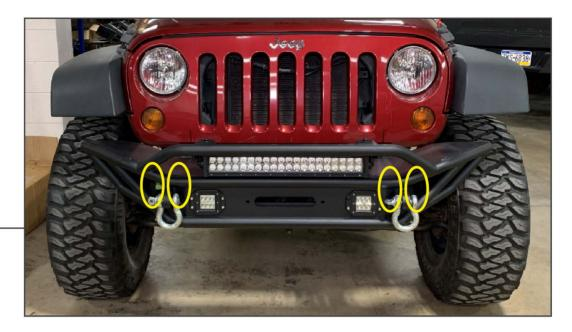
Place (2) M12 x 35mm stud plates and into the inner and outer sections of the bumper. Hold the studs in place using the (4) plastic stud holders. Add (2) bumper spacers to the outer studs. Align the bumper to the vehicle and secure to the bumper using the (4) M12 x 35mm bolts, (4) M12 nuts, (8) M12 lock washers, and (8) M12 flat washers.
