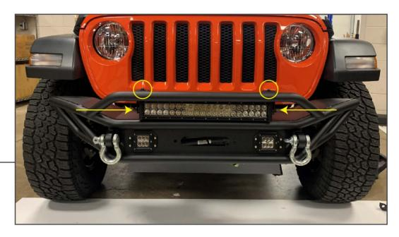
Secure the (2) light bar brackets to the bumper using (2) M8 x 25mm Allen bolts, (2) M8 lock washers, (2) M8 flat washers, and (2) M8 nuts. Secure the light bar to the brackets using (2) M8 x 16mm Allen bolts, (2) M8 lock washers, and (2) M8 flat washers. Using the provided wiring harnesses, connect the lights to the vehicle.
