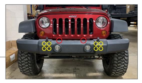
Remove (2) plastic push clips from the upper plastic trim panel behind the bumper. Unplug the fog lights from the bumper. Remove (8) 18mm nuts from the back side of the bumper. Remove the bumper from the vehicle.
