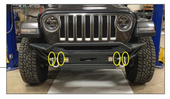
Place (4) M12 x 35mm stud plates and into the inner and outer sections of the bumper. Hold the studs in place using the (4) plastic stud holders. Add (1) bumper spacer to each of the outer stud plates. Align the bumper to the vehicle and secure to the bumper using the (4) M12 x 35mm bolts, (8) M12 lock washers, and (8) M12 flat washers, and (4) M12 nuts
