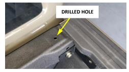
Place Rear Riser Tube on the vehicle as shown, align tube flanges to corners of the bed and Corner Brackets to locate and temporally bolt down using M8 Button Socket Bolts.
