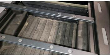
**8.** PRE-ASSEMBLE ALUMINUM PLANK ASSEMBLIES (3 PLANKS, 6 BRACKETS, 24 FLANGEDS NUTS). Bolt Plank Brackets to Aluminum Planks at one end of the planks as shown. Do it for all 3 planks. Slide 4 of M6 Flange Nuts in each channel track in the Aluminum Planks. Total of 8 Flanged Nuts per plank. Now bolt the remaining Plank Brackets to the other end of the plank to complete the Plank Assemblies.
