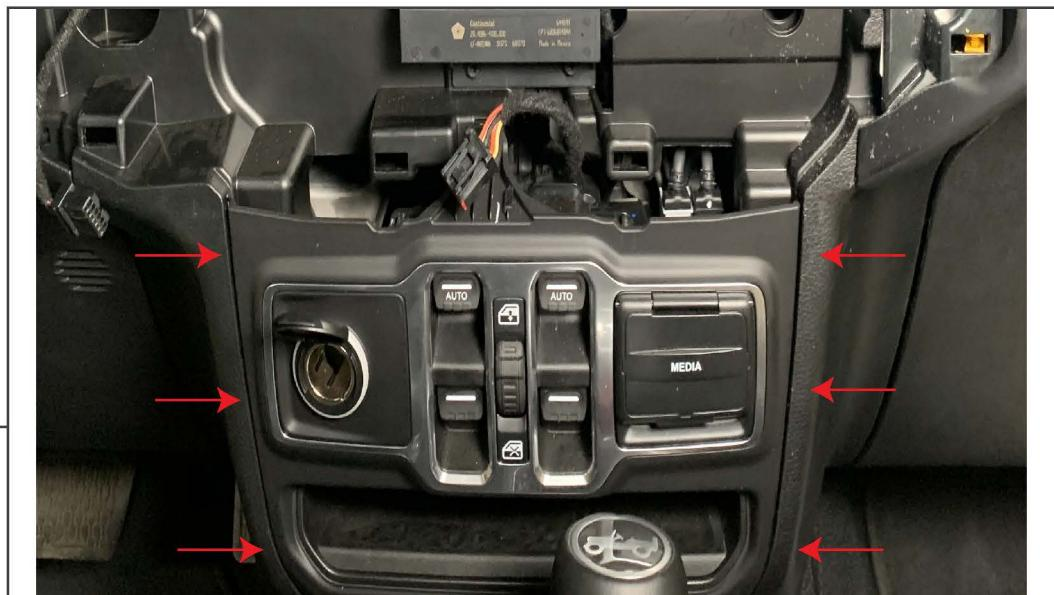
Using a panel removal tool, unclip the window switch panel from the dashboard. Unplug the 12V cigarette lighter connector.
