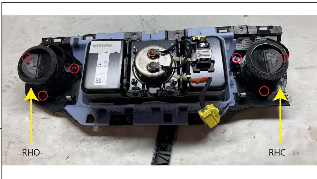
Remove (3) 7/32 screws securing the each vent to the airbag assembly. Lightly pry back on the plastic mounting tabs to release each vent from the airbag assembly. Do not mix up the vent locations.
