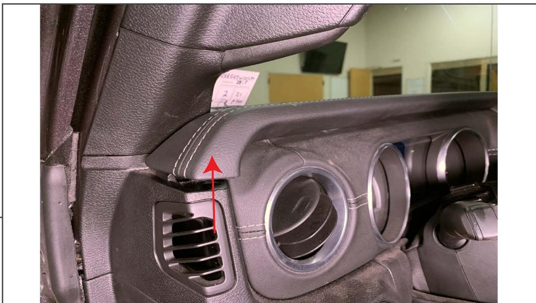
Using a panel removal tool, release the top dash pad from the dashboard. Pull the pad towards the steering wheel to remove. Do this all the way across the dashboard.
