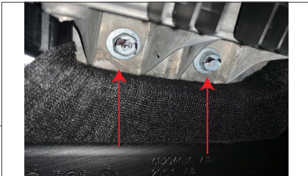
Remove glove box from vehicle by pushing up on the stopper in the middle, then lift the box away from the dashboard. Remove (2) 13mm bolts above the glove box location releasing the air bag with the vents.
