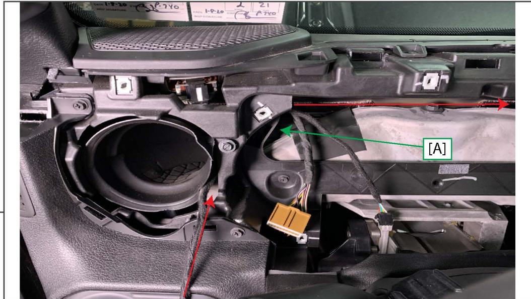
Beginning with the passenger side of the wiring harness, route the harness throughout the dashboard. Store the power module at the marked location [A].
