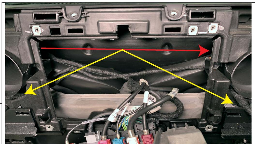
Continue routing the harness throughout the dashboard, allow the (2) center vent connectors to rest at their corresponding ducts.
