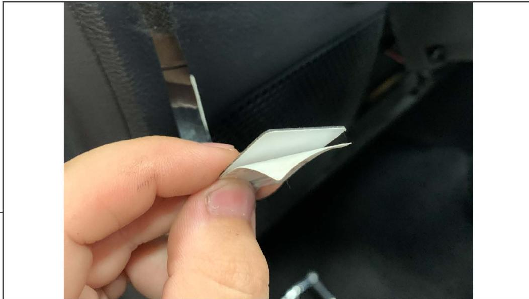
Route power switch to desired location, then using provided double sided tape, adhere to clean surface area of the dashboard.
