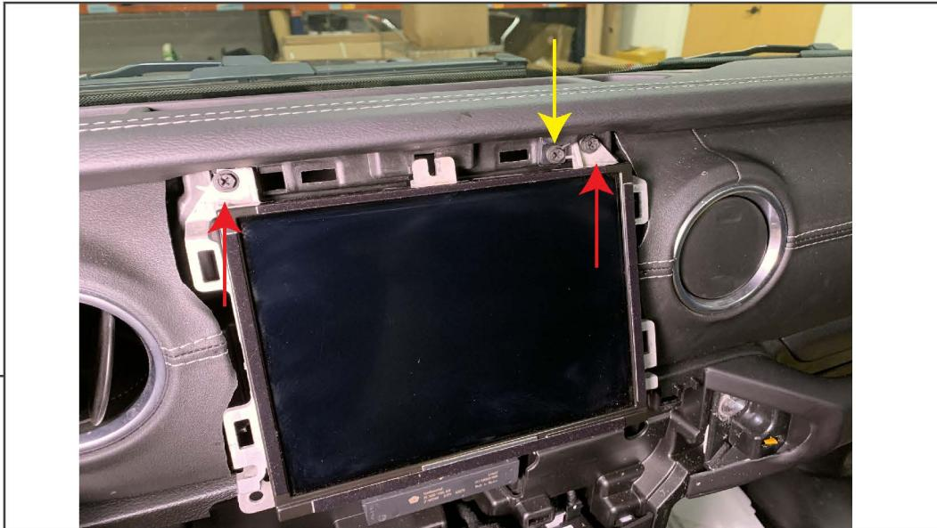
Remove the (2) Phillips screws to release the touch screen from the dashboard. Allow the touch screen to hang. Remove (1) Phillips screw from the dash pad.
