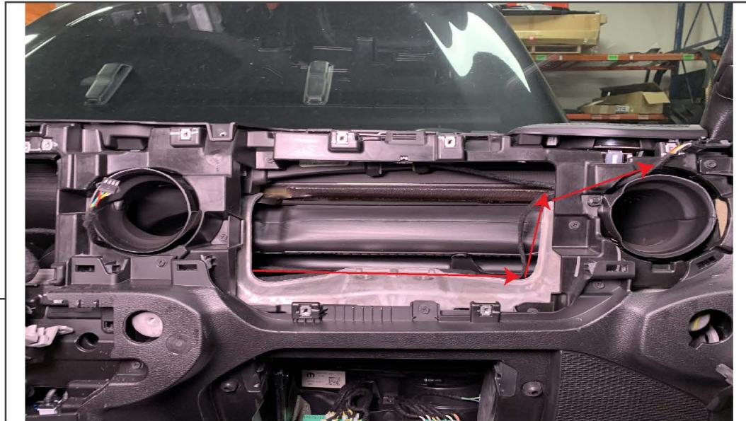
Route the wiring harness to the passenger side outer duct. Be sure to route the wiring harness neatly to prevent interference with the airbag.
