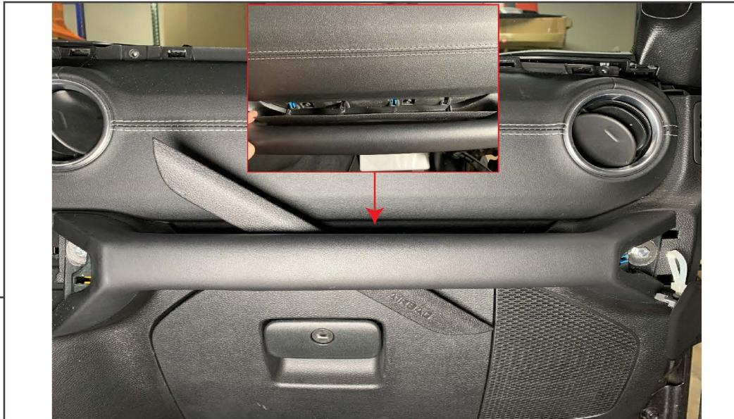
Remove the side cap from the grab handle. Remove (2) 10mm bolts to remove handle from dashboard. Remove from vehicle. Release the airbag trim panel using a panel removal tool.
