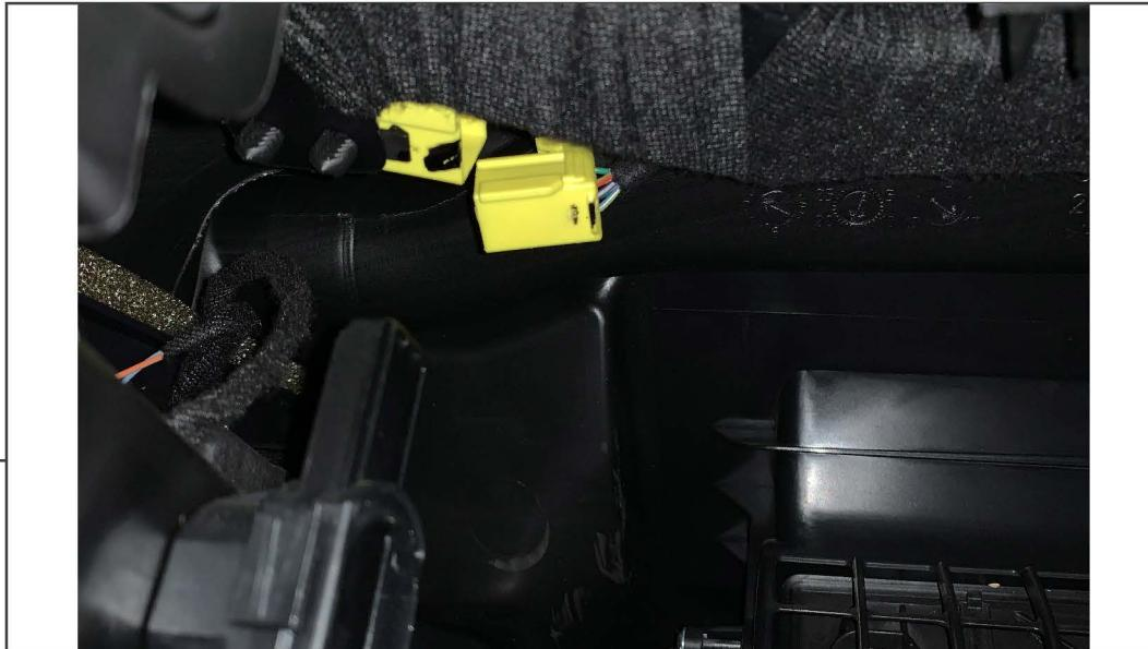
Along the left hand side of the dashboard behind the glove box location, unplug the airbag connector by pushing down on the top of the connector. Remove airbag assembly from vehicle.
