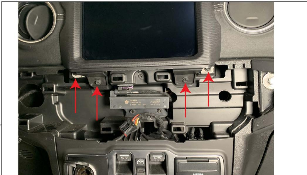
Remove (4) Phillips screws at the bottom of the touch screen bezel. Then, release the (6) clips holding the remaining three sides of the touch screen bezel to the dashboard using a panel removal tool.
