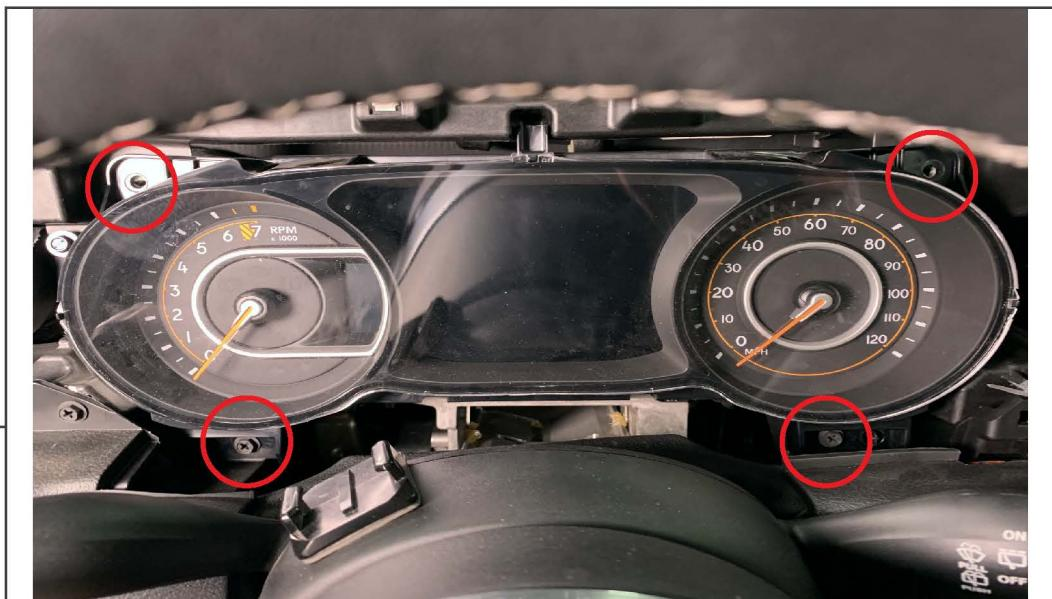
Release the clips around the steering wheel bezel and move the bezel aside. Remove (4) Phillips screws from the instrument cluster. Unplug instrument cluster from the rear and Remove from vehicle.
