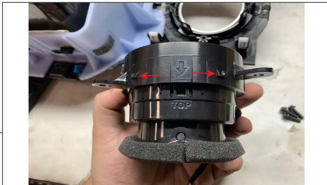
Locate [TOP] on the LED Vents as well as the appropriate location indicator. Push the LED Vent into the appropriate location with [TOP] facing up. There will be an audible click when each mounting tab is secure. Reinstall (3) original screws per vent.
