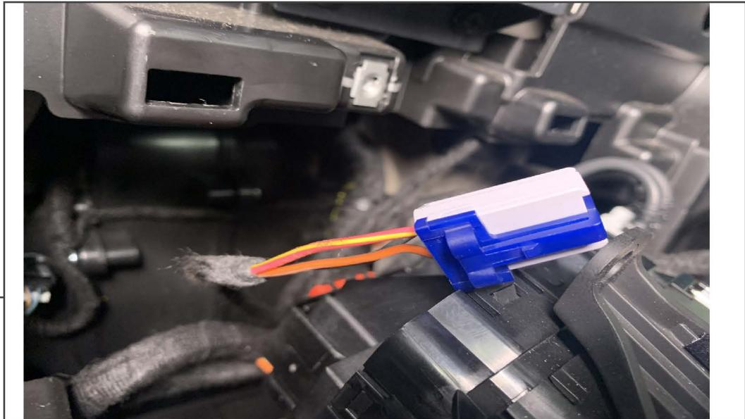
Carefully peeling back the insulation on the cigarette lighter connector, splice into the Red/Yellow wire with the Orange wire in the provided wiring harness. Cut the provided Orange power wire on the provided wire harness to length if it is too long.
