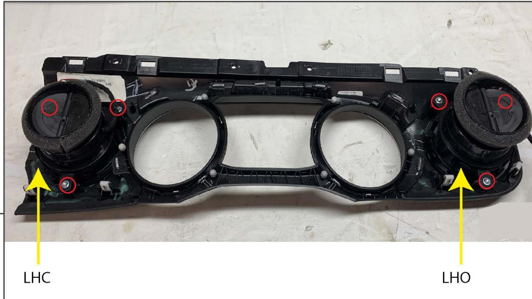
Remove (3) T15 Torx screws securing the each vent to the airbag assembly. Lightly pry back on the plastic mounting tabs to release each vent from the airbag assembly. Do not mix up the vent locations.
