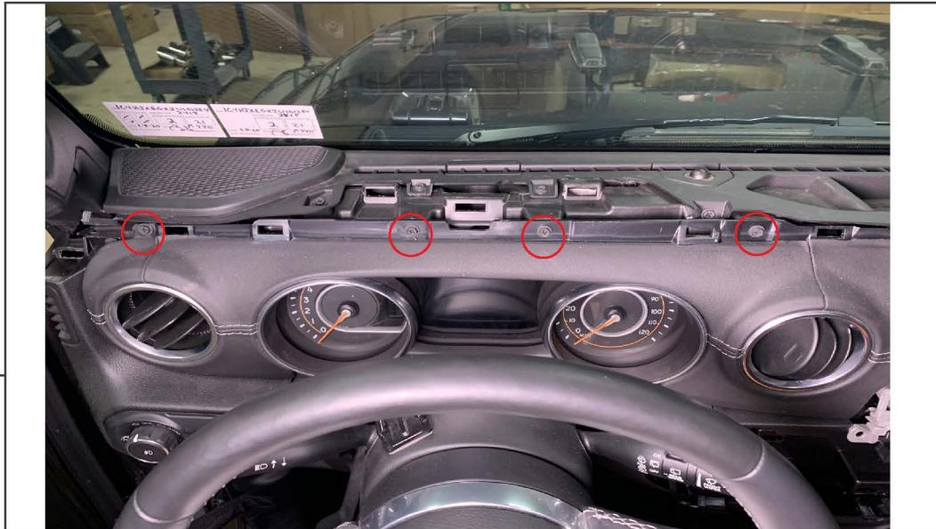
Remove (4) Phillips screws from the instrument cluster bezel. Then use a panel removal tool to release the bezel from the dashboard. Remove from vehicle.
