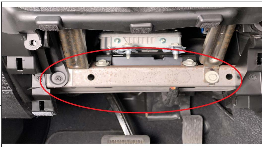
Route the provided Brown ground wire to the lower portion of the dashboard. Be sure not to route the wire in the way of any moving components.
