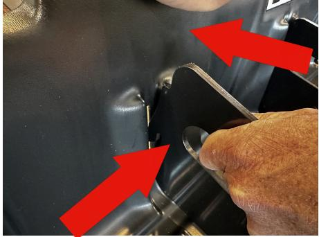
Step 2: Pull and lift up with the handle on the divider. This motion combined with pushing on the back allows for the divider to pop loose.
