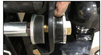
Figure 16: Hitch frame resting on bump cushions closer to trailer - stop adding air.
