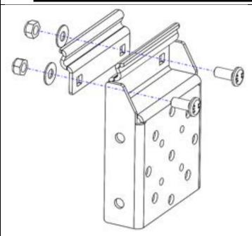
Install M8 coach head screws, washers and nyloc nuts through mount and clamping bracket as shown.
