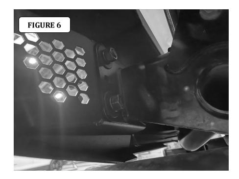
**Step-17** Attach the bumper bracket to the frame horn using (1) 3/8" x 1 1/4" hex bolts, (2) 3/8" flat washers, (1) 3/8" lock washer and (1) 3/8" hex nut. Leave the nuts and bolts loose for final adjustment.
