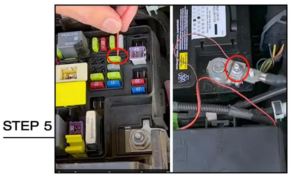
Open the fuse box, connect the red wire to the ACC, the black wire to the negative terminal.
