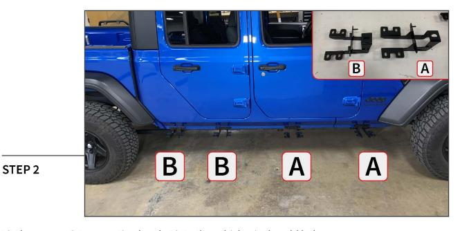
Fit the appropriate mounting bracket into the vehicle pinch weld holes.
