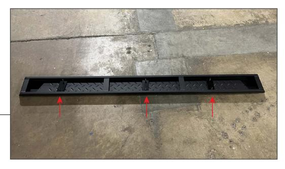
Fit (3) stud plates onto the inside of the side step. Then, fit the side step to the brackets, ensuring the studs align within each mounting bracket.
