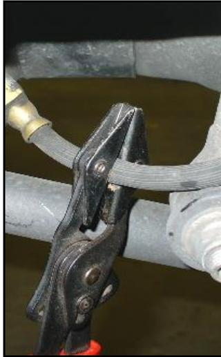
**Figure 1:** Hose crimper applied to OE brake hose
