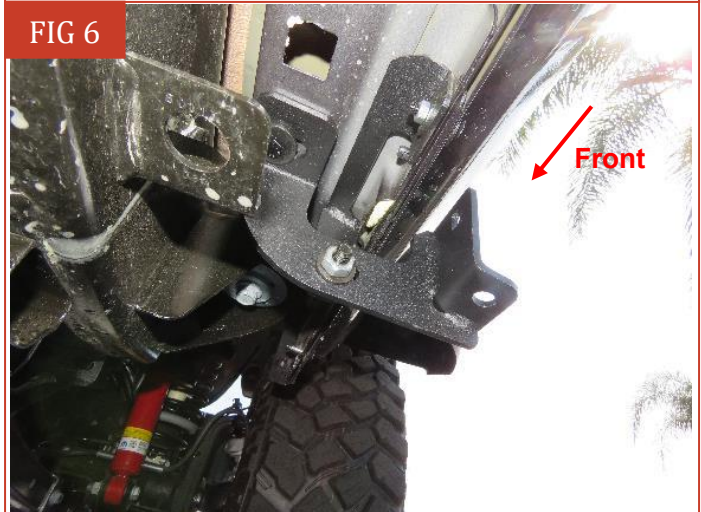
(Fig 6) Passenger/Right front mounting bracket and support bracket attached.
