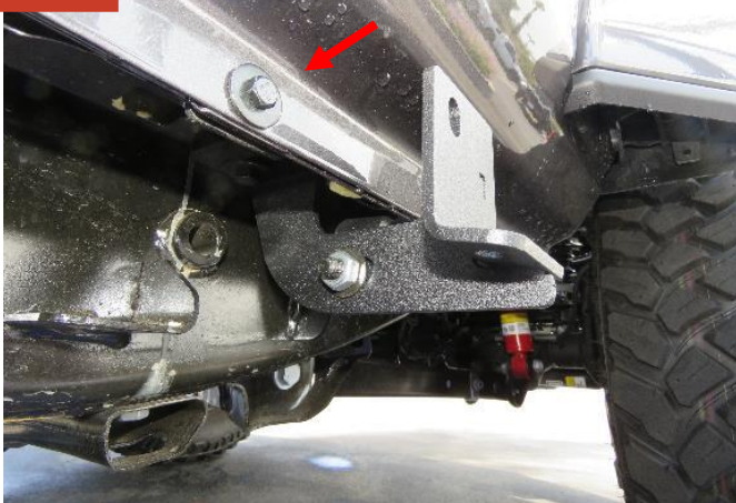
(Fig 4) Insert Bolts from the outside of the pinch weld.
