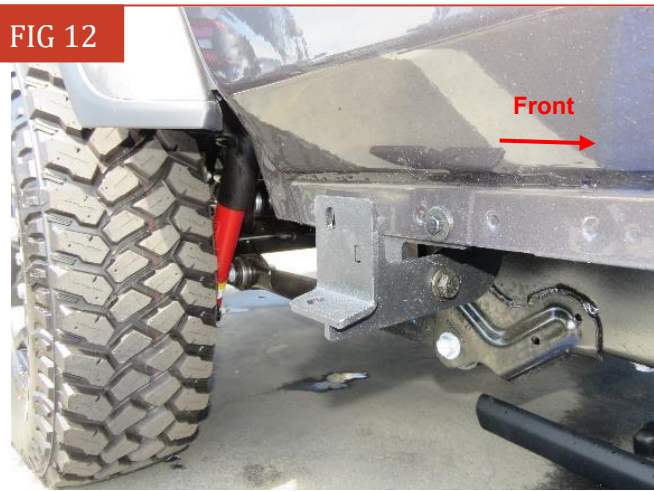
(Fig 12) Attach Passenger/Right Rear Bracket and Passenger/Right Rear Support Bracket to the rear location
