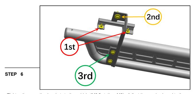
Tighten the mounting brackets to the vehicle (M6 first, then M8). Adjust the running board to the desired angle, and tighten the M8 combo bolts to secure the step into place. See photo for tightening order visual.
