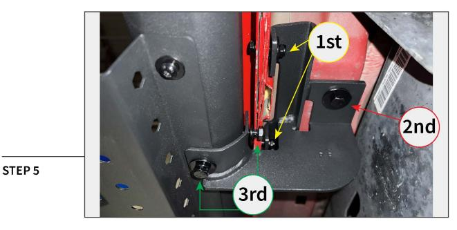
Adjust the running boards and bracket for the desired fit to the vehicle. Tighten all hardware following the diagram above.
