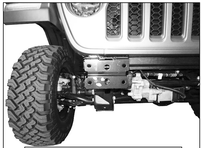
(Fig 7) Front Bumper and splash guard removed (2020 Gladiator JT shown)
