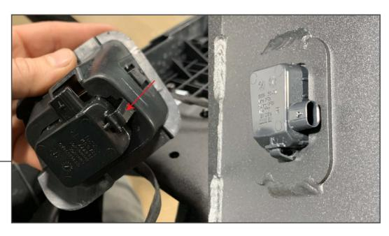
With the license plate housing separated, depress the tab on the light and remove it from the housing. Transfer the light to the new bumper. Transfer the wiring harness from the stock bumper to the new bumper.
