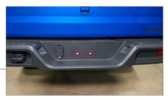
Remove the license plate to access the remaining (2) 16mm bolts securing the bumper to the vehicle. Carefully remove the bumper and rest it on a soft surface.
