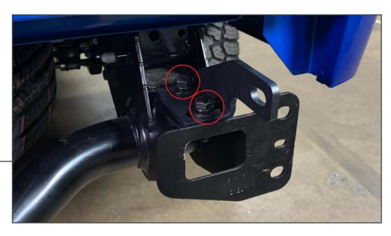
Loosely mount the additional bumper brackets to top of the frame rail using (2) M12 bolts, (4) M12 washers, (2) M12 lock washers, and (2) nuts per bracket.
