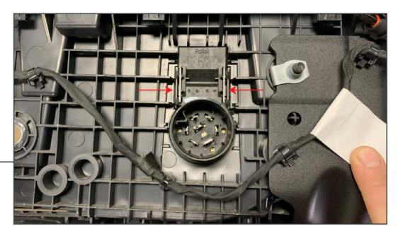
Depress the clips securing the trailer wiring plug and press the connector through the bumper. Transfer the plug on to the new bumper.
