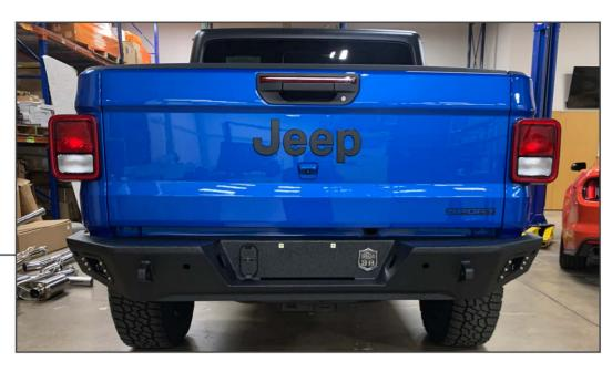
Remove the bumper wiring harness from the factory bumper and transfer it to the new bumper. Plug it in to the license plate lights and trailer wiring plug. Press in the plastic license plate screw retainers and install the license plate to complete the installation.
