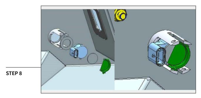
Optional Sensor Mounting: Place the round foam on the back of the sensor. Press the sensor into the bumper. Then clip the retaining plate onto the bumper to hold the sensor in place.
