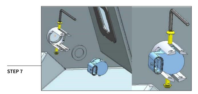
Optional Sensor Mounting: Using the provided M4 Allen screws lightly tighten the screws into the sensor to hold it in place. \*\*Note: Over tightening the screws can damage the sensor.
