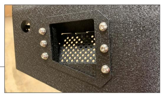
Install the bumper bezels using the provided Allen wrench and (6) Allen bolts, (6) lock washers, and (6) flat washers per side.
