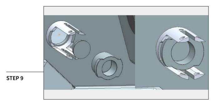
No Sensor: Mount the hard rubber plug to the front of the soft rubber plug. Press the assembly into the bumper so that the hard rubber plug is flush with the face of the bumper.
