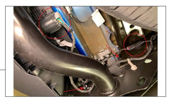
Located at the left rear of the vehicle, behind the bumper, begin by disconnecting the trailer plug wiring harness. Then disconnect the license plate wiring. Free the wiring from any wiring clips securing the wiring to the bumper or bumper brace.
