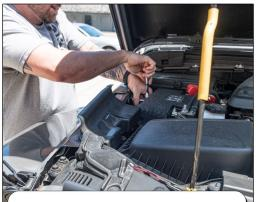
Route the black wire along the passenger fender to the ground post. Ground post is a 10mm bolt.
