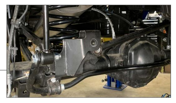
Lower the vehicle to the ground with the wheels installed. With assistance, gently push the vehicle body to allow the track bar to properly align with the axle. Then, secure the track bar to the axle using the original (1) 21mm bolt & nut.
