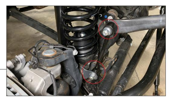
Secure the (1) front sway bar link to the vehicle sway bar and axle using (2) M12x1.75 x 65mm bolts, (2) M12 flat washers, and (2) M12 locking flange nuts.
