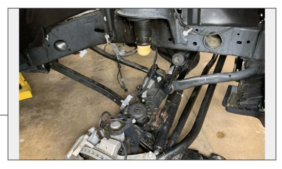
Lower the floor jack to relieve tension from the coil spring. Once the spring is relieved of all tension, lift and remove the spring from the vehicle.
