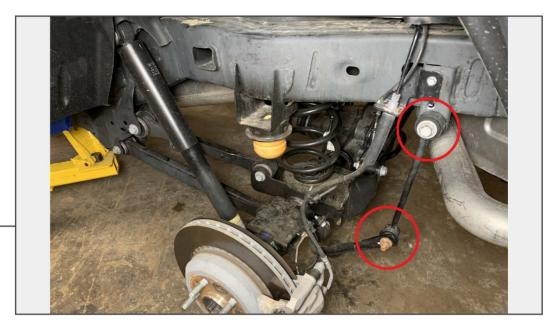
Remove the (1) 18mm bolt and (1) 18mm nut to remove the sway bar link from the vehicle.
