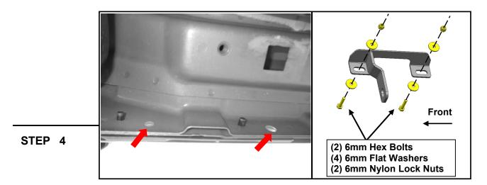
Loosely fit the Passenger Front reinforcement bracket to the inside of the vehicle pinch weld using (2) M6x25mm bolts, (4) M6 flat washers, and (2) M6 lock nuts. Do not fully tighten to allow for later adjustments.
