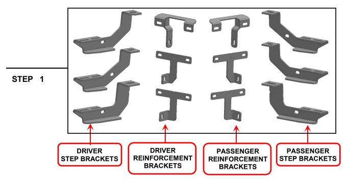
Mounting Brackets and Reinforcement brackets look very similar but are unique. Please identify each mounting bracket using the engraved location identifier.
