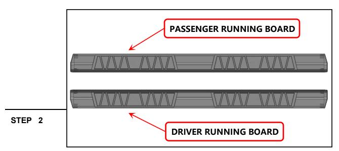
Identify each Running Board by the front of the step. Notice: "D" for Driver/Left Side; "P" for Passenger/Right Side.
