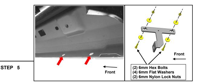
Loosely fit the Passenger Center reinforcement bracket to the inside of the vehicle pinch weld using (2) M6x25mm bolts, (4) M6 flat washers, and (2) M6 lock nuts. Do not fully tighten to allow for later adjustments.
