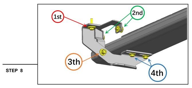
Tighten the mounting brackets to the vehicle. Adjust the Running Board to the desired angle, and tighten the M8 combo bolts to secure the step into place. See photo for tightening order visual.
