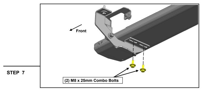
With all brackets loosely mounted to the vehicle, fit the Running Board onto the brackets, and loosely secure into place using (6) M8 x 25mm combo bolts.
