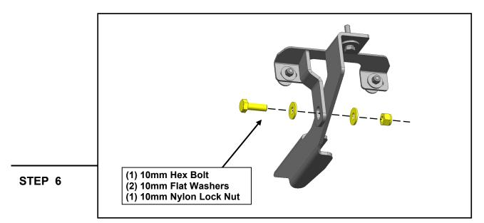
Loosely attach the (1) Passenger Front step bracket to the (1) Passenger Front reinforcement bracket using (1) M10 bolt, (2) M10 flat washers, and (1) M10 nylon lock nut.
