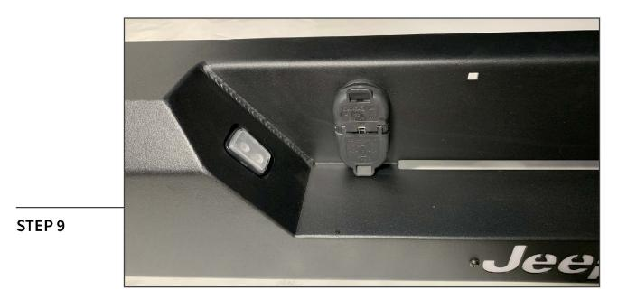
Firmly press the trailer wiring connector into the bumper until fully seated.
