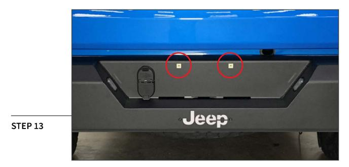
Press the (2) license plate screw retainers into the rear bumper.
