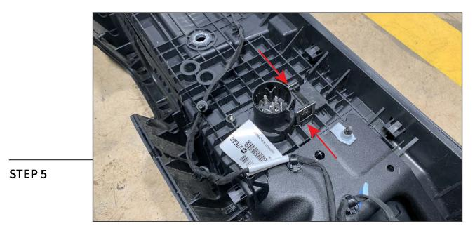
Using a pry tool, press each side of the trailer wiring connector, and remove the connector through the front of the bumper.
