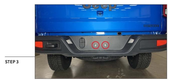
Remove the license plate from the vehicle, then remove (2) 16mm bolts from the bumper. Lift and remove the bumper assembly from the vehicle. Place on a soft workable surface for disassembly.
