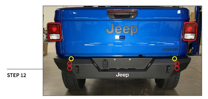
With assistance, lift the bumper to the vehicle frame rails and secure using (4) M12 flat washers, (4) M12 lock washers, and (4) M12 nuts. Then, secure the upper bracket to the bumper using (2) M12 x 40mm bolts, (4) M12 flat washers, (2) M12 lock washers, and (2) M12 nuts.
