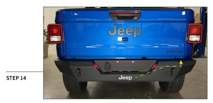
Neatly route and plug in each license plate lamp using the original wiring harness. Then, plug the included wiring harness into the Jeep logo backlight.
