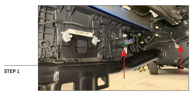
Under the vehicle, unplug the license plate lamp wiring harness and the trailer lighting connector harness.
