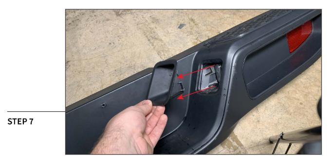
Use a plastic pry tool to remove the outer license plate covers. Then, remove the license plate lamp through the back of the bumper.
