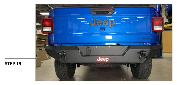
Ensure all bumper hardware is fully tightened, and the wiring harnesses are neatly routed away from any moving/hot components. Install the (2) 3/4" D-Rings into the bumper mounting points.
