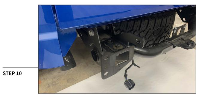
Install the upper mounting brackets to the vehicle frame using (2) M12 x 40mm Bolts, (2) M12 flat washers, (2) M12 lock washers, and (2) M12 nuts. Do not fully tighten at this time.
