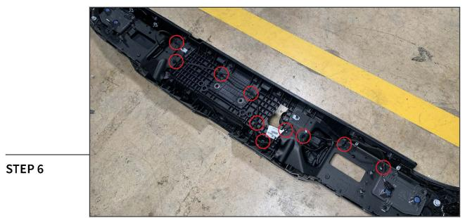
Unplug each license plate lamp from the original bumper, and use a panel removal tool to disconnect the plastic clips securing the wiring harness to the bumper. Set wiring harness aside.
