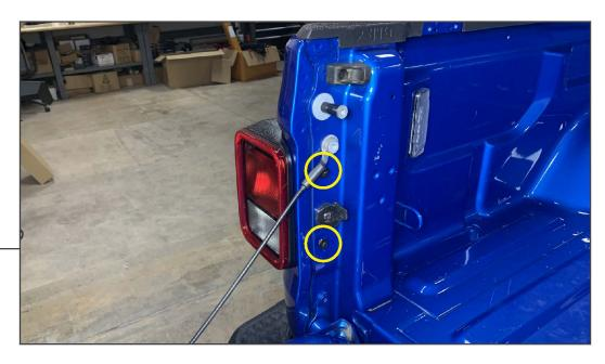
Lower the tailgate to access the tail light bolts. Using an 8mm socket, remove the (2) bolts securing the tail light to the vehicle.
