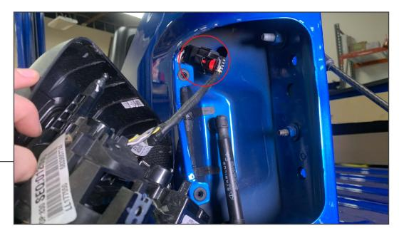
Slide the red lock tab back. Depress the tab on the electrical connector while pulling the connectors away from each other.
