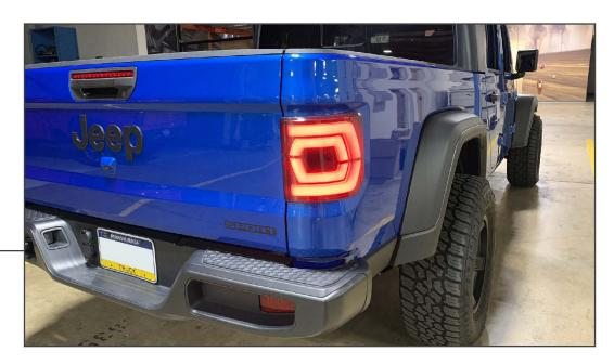
Push the tail light into the vehicle, ensuring the alignment pins align to the rubber grommets within the bed. Secure the tail light using the OEM bolts.
