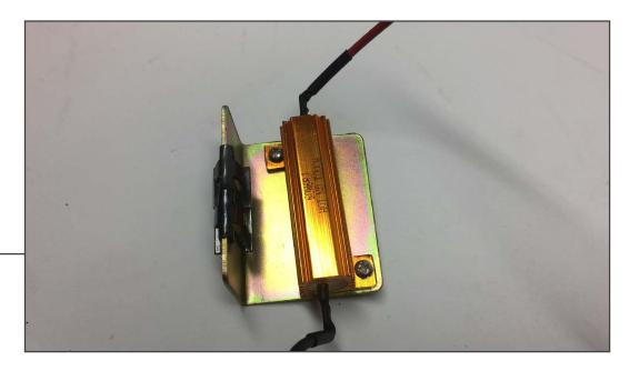
Install (2) metal clips to the resistor bracket.
