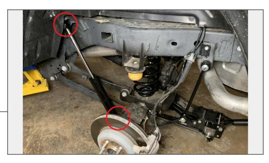
Install the new rear shock absorber to the vehicle using the original (2) 21mm bolts & nuts.
