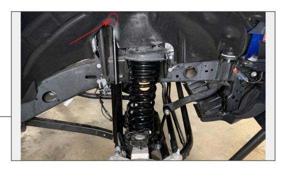
Ensure the coil spring rubber isolators are still installed to the vehicle frame and axle. Then, fit the coil spring into the vehicle, ensuring the spring is properly turned to fit into the lower isolator groove.
