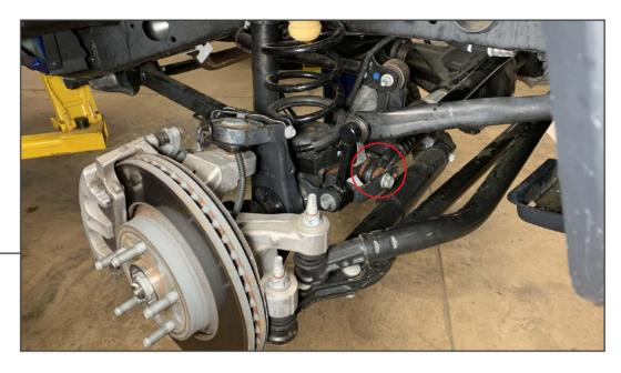
Remove the 21mm bolt securing the track bar to the axle.
