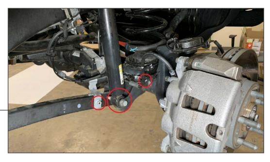
Remove the 18mm lower shock mounting bolt from the axle. Remove (1) 10mm bolt from the brake line bracket under the spring perch. Remove (1) 15mm nut from the brake line bracket attached to the lower control arm.
