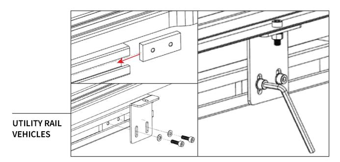
Remove the rail end caps from the utility rails. Slide each bracket onto the utility rail. Use the provided hardware to secure the tonneau cover bed rails to the utility rails. Install all hardware loosely at first, then position the bed rails into place. Once positioned, tighten the upper bolt into place, following with the lower utility rail hardware.
