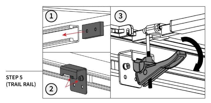
**Trail Rail System:** Slide the (2) bolt plate block portions of the bed track clamps into the Trail Rail system. Once spaced evenly, use (2) Allen bolts per block plate and secure the mounting bracket.
