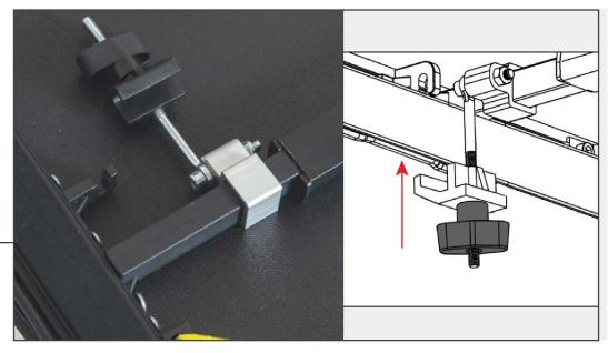
Once aligned, carefully fold the tonneau cover up towards the cab of the vehicle to access the (2) front pre-installed folding clamps. Slide the clamp rod to the appropriate distance, then fit the hook under the metal bed side. Thread the thumb screw upwards to tighten the tonneau cover to the front of the vehicle bed. \*\*See Step 6 for Trail Rail System mounting.
