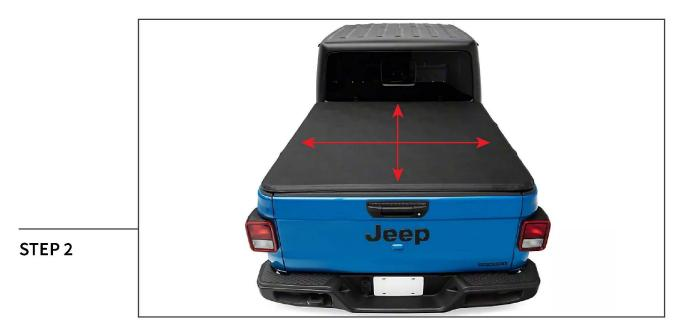
Fold the tonneau cover outwards towards the rear of the vehicle. Adjust the tonneau cover forward/backwards and left/right until proper adjustment is achieved.
