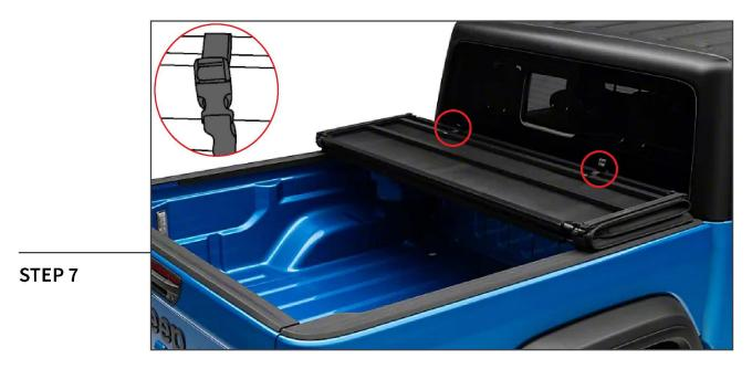
To store, undo the (2) rear clamps, and fold the tonneau cover towards the vehicle cab. Insert the rear clamps into the under side of the cover. Secure the tonneau cover to the attached straps and buckles.
