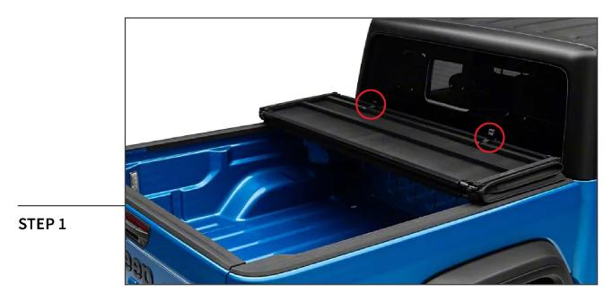
Place the tonneau cover onto the vehicle bed closest to the cab. Ensure the panel retaining strap clips are closest to the cab.
